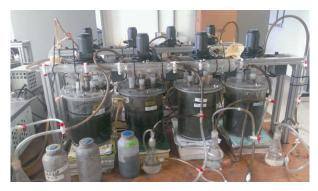
Figure 2. Eight bench-top 3-L completely stirred tank reactors were set-up with condition of 5% or 8% total solids coupled with 37°C or 55°C incubation temperature. Each condition was started-up with duplicate anaerobic digesters for further long-turn observation.
